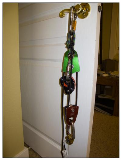
of my 2:1 setup. I was trying to go light by using a Ropeman in place of a Basic but ended up not liking how it worked and changed back to the Basic.
