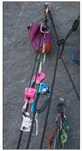
coming from. If there was no Universal, the "Zed Cord", the cord that runs through your pulleys, would grind on the edge of the top pulley and you would loose efficiency. The Zed Cord can be 5 mil Spectra cord, but be careful, Spectra cord is pretty delicate and can easily abrade and break on one route. There is a new kind out, I don't know it's name but it doesn't stretch and resists abrading far better. You'll want Spectra because it is strong and doesn't stretch.
